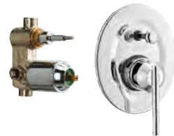
High flow single lever concealed diverter system consisting of Exposed part (lever, tip ton knob, flange) and Concealed part (45 mm cartridge with button assembly, cartridge sleeve)
