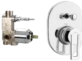
5-way (3 inlets + 2 outlets) single lever concealed diverter system consisting of Exposed part (lever, tip ton knob, flange) and Concealed part (cartridge with button assembly, cartridge sleeve)
