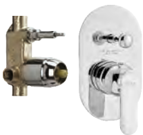
Single lever concealed diverter system consisting of Exposed part (lever, tip ton knob, flange) and Concealed part (40 mm cartridge with button assembly, cartridge sleeve) Exposed part F1018701 ₹ 2410 Concealed Part F4010101 ₹ 3445 Set ₹ 5855
