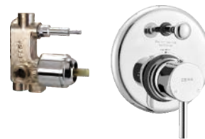
5-way (3 inlets + 2 outlets) single lever concealed diverter system consisting of Exposed part (lever, tip ton knob, flange) and Concealed part (cartridge with button assembly, cartridge sleeve)
