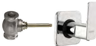
Stop cock consisting of exposed part (sleeve, lever, wall flange) and concealed part suitable for 15 and 20 mm pipeline with inner head
